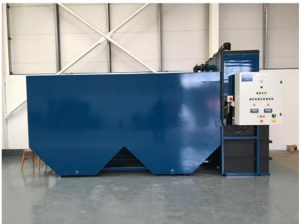
The control system on the unit with automatically dose the contaminated water until the pH is within safe levels, only when the levels are within the pre set parameters will the solenoid open to send the water to drain. We set the parameters based on the limits given by your local water authority. The control panel has warning alarms to advise an operator of an issue, if the levels re not met the solenoid will not open and it will re treat the water until it is within the required levels.
