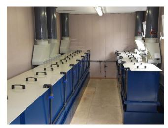
This line was a manual acid etch and passivation line. We included all equipment such as heating, thermostats, agitation, lids, pipework and fume extraction. This line was fitted into a container to save space in the main factory and the fume extraction was mounted on the roof.
