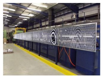
The transporter will move along the plant into each tank. The extraction hoods run along the length of the tank rather than at the rear.
