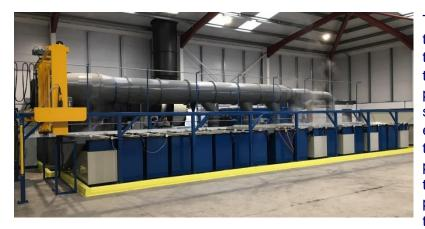
This line was fully automated, with the transporter moving the jigs along the line and into each tank to avoid the need for an operator to manually process. We included all equipment such as heating, thermostats, eductor agitation, rectifier, chiller, transporter, control panel with auto plc, fume extraction and waste water treatment plant. This line is protected with a light beam along the operator side and in the
