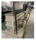
We place pumps and pipework and electrics at the rear of the line to keep the front walk way clear for the operators, but this allows access for maintenance. All equipment is inside the bund tray in case of leaks. This line is fully automated with transporter, and all ancillary equipment required. This has traditional metal guarding along the operate side for safety, this is instead of a light beam.
