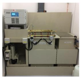
This plant was a compact Copper electroforming unit, it including the Copper tank and a rinse tank. Due to limited space we designed the unit to have the filter pump in a bund tray on the floor with the agitation motor and rectifier mounted above. passivation line. We included all equipment such as heating, thermostats, pipework and fume extraction.
