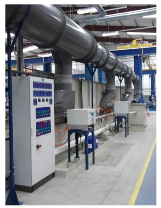
We place pumps, pipework and electrics at the rear of the line to keep the front walk way clear for the operators, but this allows access for maintenance. In this instance the customer also opted for the control panel, the rectifiers and a pH correction tank to be at the rear of the line as well. We will work with you to make use of the space you have available and suggest the most practical layout.
