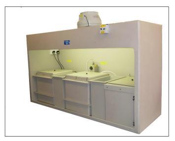
This line was a manual line for electropolishing of Stainless Steel. Due to restrictions on space it could not be positioned in on long row, so it was placed in an "L" shape. This allowed the rectifier to be positioned in the corner to make use of the space and all eductor pumps and pipework were hidden at the rear in a bund tray.
