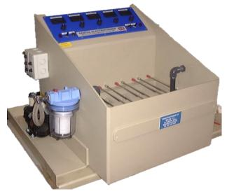
Detail view of the EFORM 10X model showing individual power supplies to 5 pairs of cells. Continuous filtration via a polypropylene cartridge prevent the nodulation of the workpiece from foreign particles plus giving an excellent structure to the deposited Silver.
